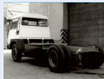
Bodyworks of an electric collection vehicle, 1974.
